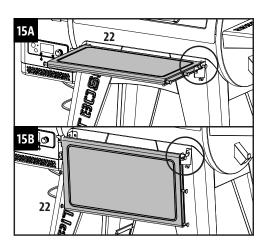
Front Shelf can also be placed on the Bottom Support Plates and be used as Bottom Plate. Note illustration 15C.
